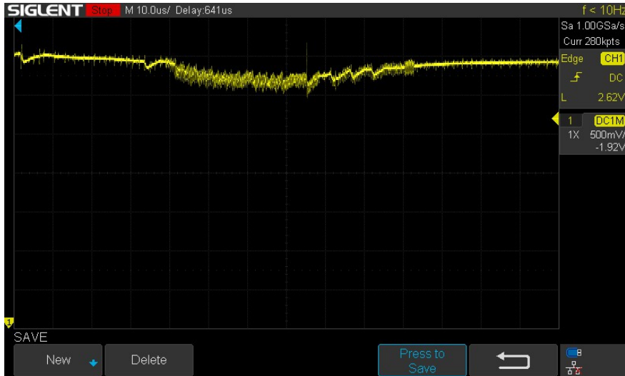
Figure 4: Successful glitch pulse at the end of the critical section (short pulse at 75\mu s in this sample)
